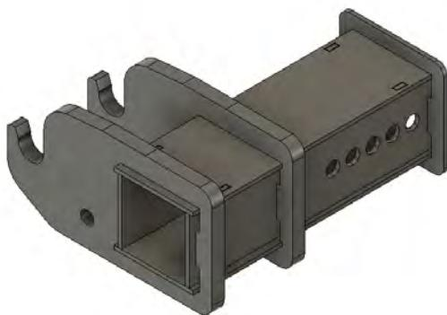
Brackets are tubes that slid over the T-bar, which is mounted on the arm of the recovery system. Different brands or types of recovery systems have different sizes of the T-bar. Dutch Recovery System offers the possibility to produce and deliver the correct dimensions for your recovery system in-house. The brackets are open on both sides, allowing them to be placed on the T-bar on both the left and right sides. The locking pins must be applied at all times.
