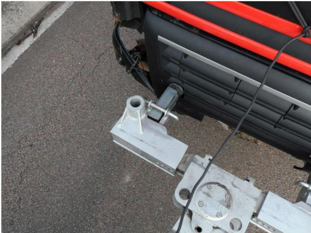
Tow hook coupled to lifting bracket, with locking pin in place
