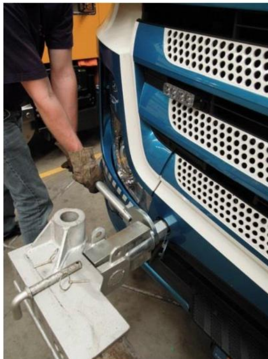
Tightening the half nut after coupling
