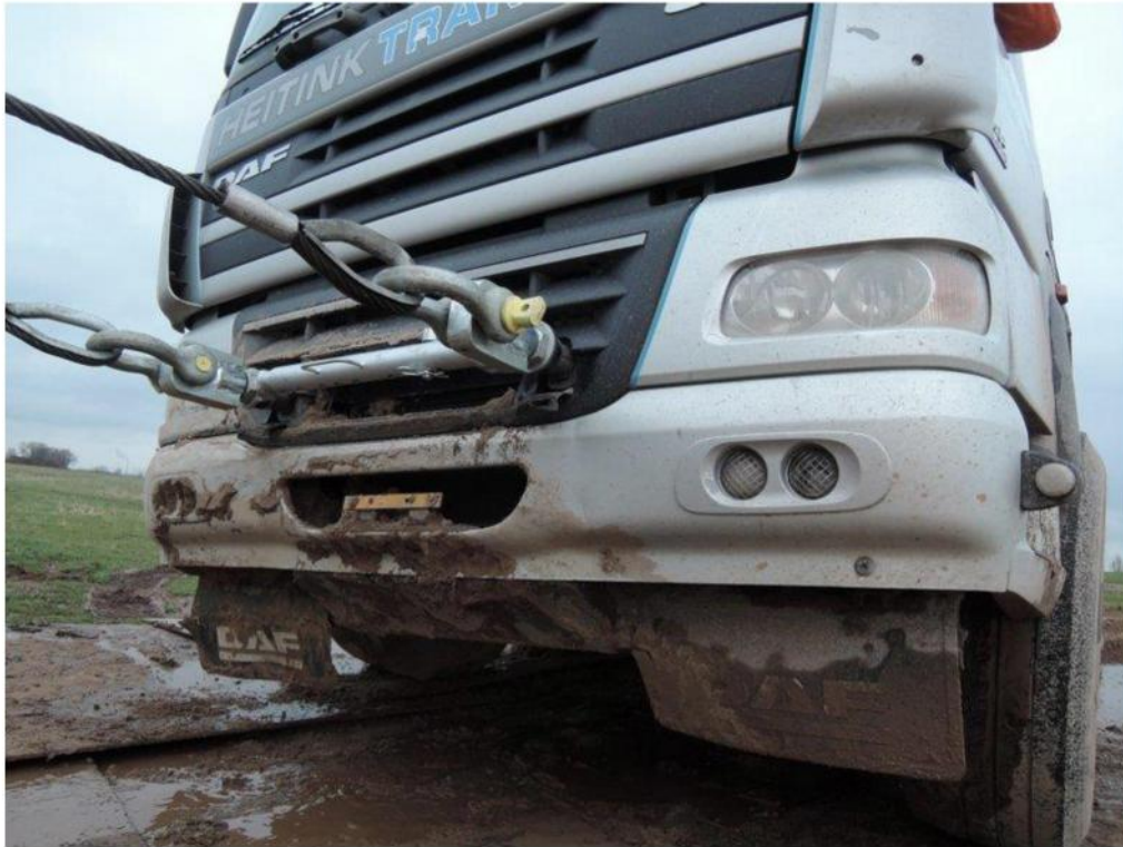
Winching with cables and winch eyes
